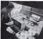
David Hunt wind-tunnel testing a third-year model with the help of a BBC Microcomputer
